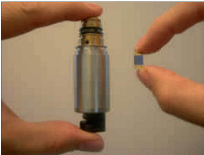
Fig. 4. Direct acting microvalve in comparison to a typical automotive solenoid valve.
