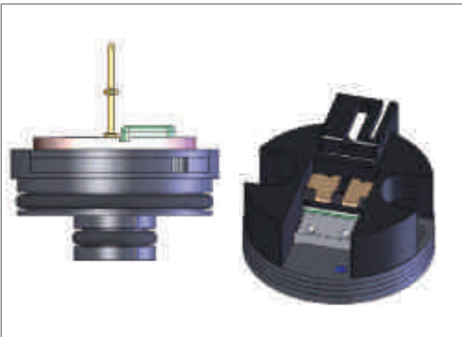
Fig. 6. (a) Microvalve piloted spool with a U-flow installation. External electrical connection and conventional cylindrical bore with o-ring seals. (b) Microvalve piloted spool with a U-flow installation. Conventional connector on a flat plate manifold using a face seal and integral filter element.
